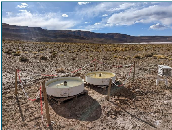
Figure 31: Evaporation test facility – brine (right) and salt water (left)
