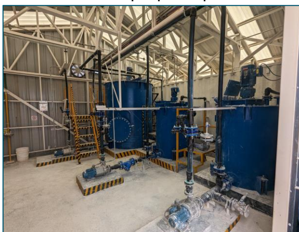
Figure 28: Reagent plant – uses Ca 2 O to lift pH from 6.2 to 10.5-11.0 to precipitate impurities
